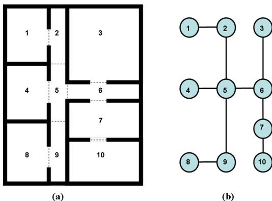
Fig. 1. Reducing a floorplan to a graph.
